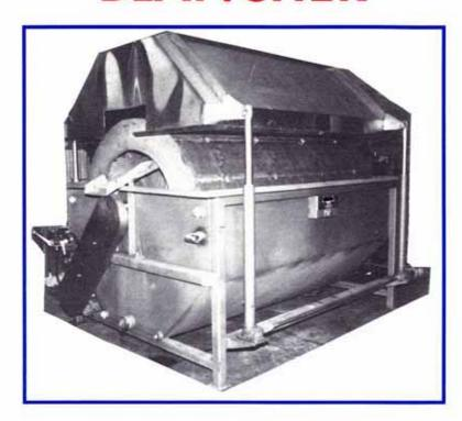
Equipped with a 230/460 Volt, 60Hz., 3 Phase, 5HP electric motor which drives a hydraulic pump, which in turn drives the cylinder through a hydraulic motor.
