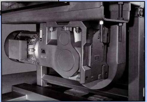
A gear type drive motor is used and drives the cage of rolls using a cog belt. A single speed gear drive is included and an AC inverter must be used.
